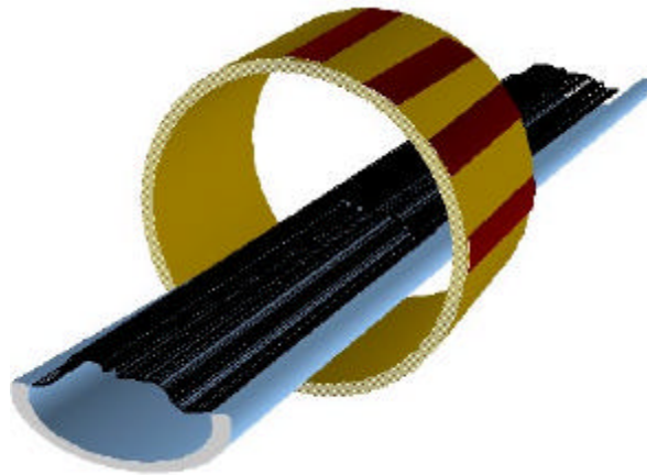
Figure 1: Schematic diagram of laboratory capacitance electrode sensor installation around a section of a narrow rubber conveyor.
