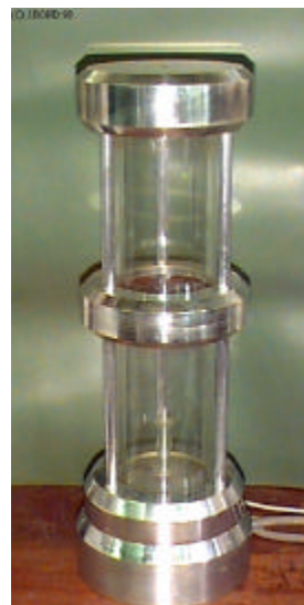
Figure 6 Bubble column with 16-electrode single plane sensor in centre of vessel
