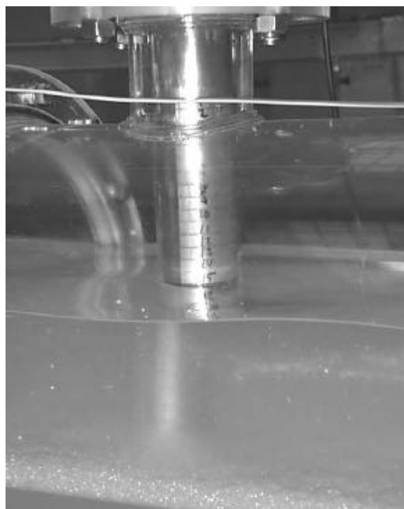
Figure 3: Photograph of probe mounted in vessel. Each electrode is numbered. An emulsion layer is seen between the condensate layer and the water layer.
