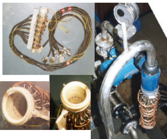
Figure 2: Examples of photographs illustrating the installation of multiple electrodes into a 50 mm hydrocyclone used in laboratory evaluations
